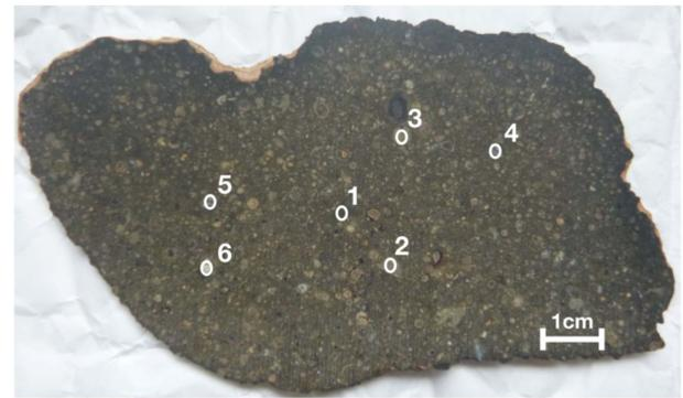
**Fig. 17.** Picture of the CV meteorite anoted with the locations of the illumination spot for the six reflectance spectra. The size of the circles represents approximately the size of the illuminated area.
