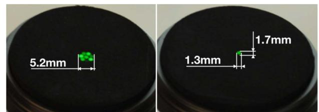
**Fig. 4.** Picture of the nominal illumination spot (left) and of the reduced illumination spot (right) of SHADOWS on a 2% Spectralon, seen from a emergence angle around  $40^{\circ}$ .
